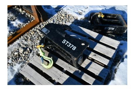
Attachments: 2020 JLG Telehandler Coupler Mounted Lift Hook
