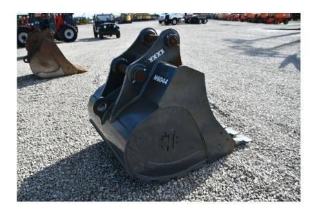
Attachments: TAG 48" SK210/SK235SR/SK230SR/SK270SR Excavator
