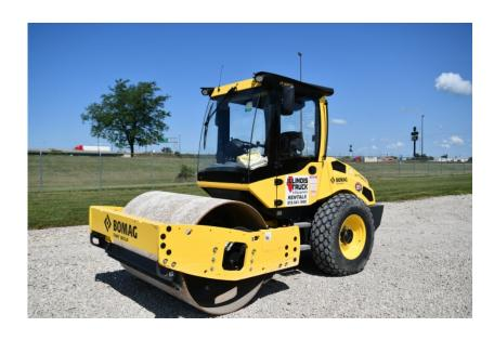
Compaction Equipment - Smooth Drum: 2017 Bomag BW177D-5
