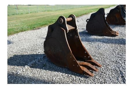
Attachments: TAG 24" SK210/SK235SR/SK230SR/SK270SR Excavator Bucket
