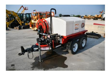
Water Equipment: 2018 Multiquip WTE5HP Water Trailer
