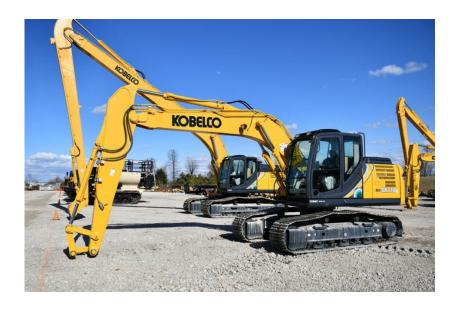
Excavator: 2020 Kobelco SK170LC-10 w/Heavy Counterweight
