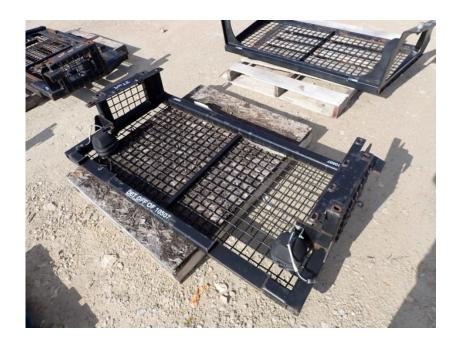
Attachments: CAT D6T Rear Window Cab Protection Screen
