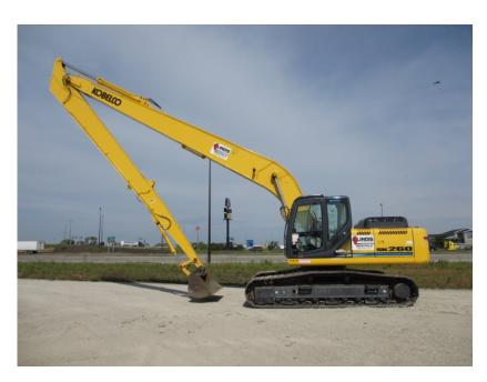
Kobelco Long Reach Excavators: Kobelco SK260 LR
