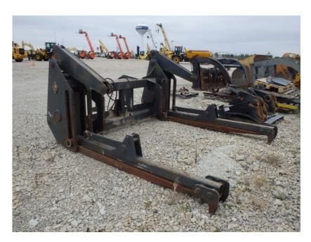
Wheel Loader Attachments: Pipe Clamp Forks: ZW150/ZW180
