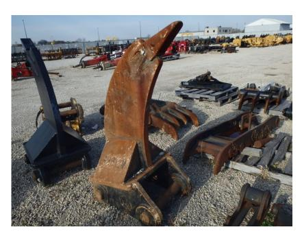
**Excavator Frost Ripper Attachments:** SK300-SK350
