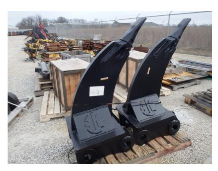
**Excavator Frost Ripper Attachments:** SK210-SK235
