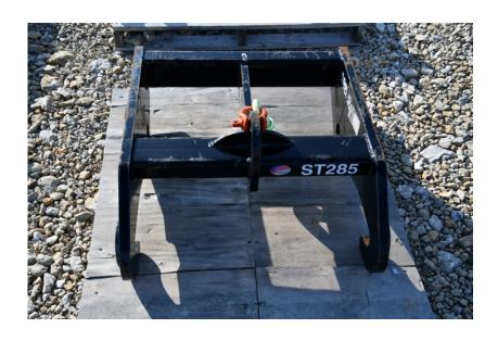
Attachments: 2018 JLG Telehandler Coupler Mounted Lift Hook
