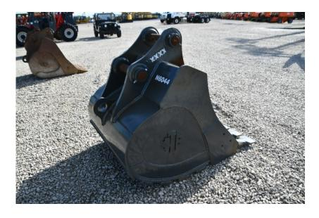
Attachments: TAG 48" SK210/SK235SR/SK230SR/SK270SR Excavator
