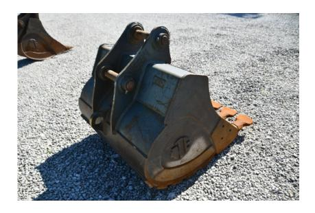
Attachments: TAG 48" SK140/SK135SR/SK130SR Excavator Bucket
