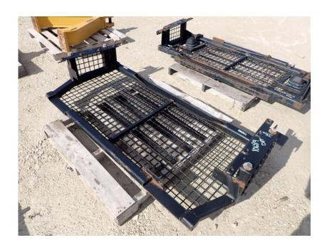
Attachments: CAT D8T Rear Window Cab Protection Screen
