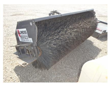
Backhoe Loader Attachments: FFC/Sweepster\* 8' Angle Broom
