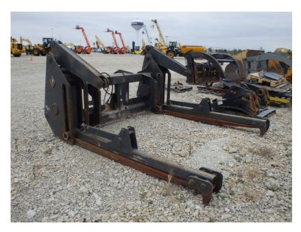
Wheel Loader Attachments: Pipe Clamp Forks: ZW150/ZW180
