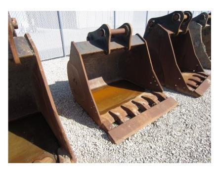
**Excavator Bucket Attachments: SK210-SK260**
